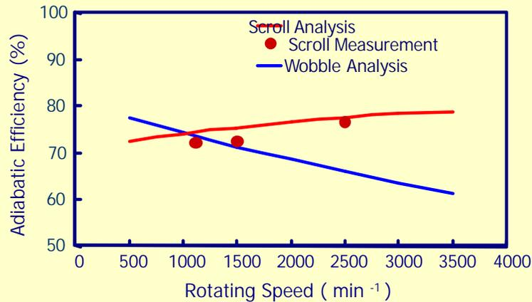
Scroll has higher efficiency especially in high speed because of no suction valve and less pressure drop.
