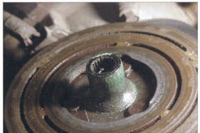
This clutch was removed from the Ford F-150 truck compressor. Sealer buildup on the clutch hub was substantial.
