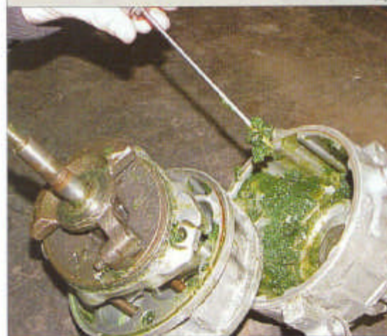
Internal compressor contamination.
