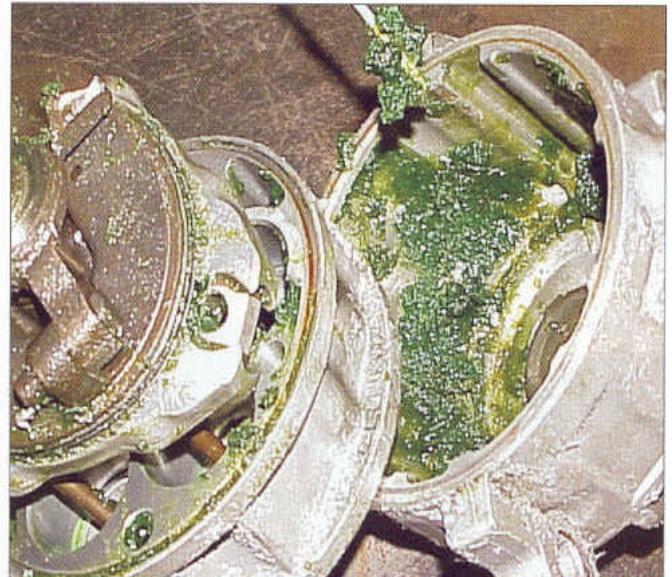
This compressor was disassembled and found to be full of green gel after return for warranty adjustment.
