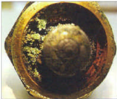
End view of solenoid valve from a recovery/recycling machine shows plugging with hardened sealer.
