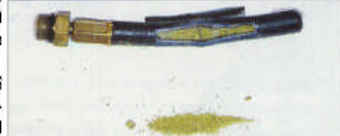
When this service hose from a recovery/recycling machine was cut open, it was found plugged with hardened sealer material.
