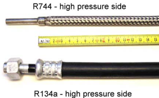
figure 6: Comparison of the geometries of a R134a and a R744 A/C hose
